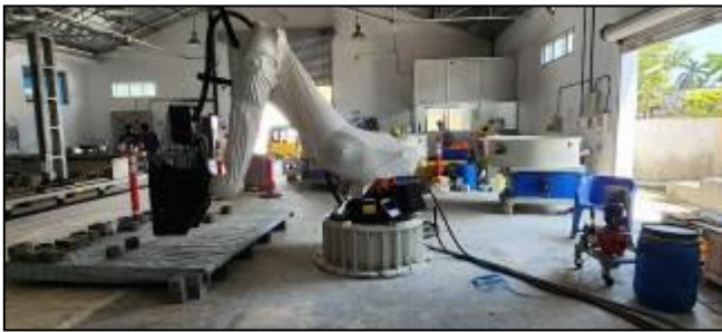
Fig -6: TVASTA’s robotic arm printer at TVASTA Factory at OMR – Chennai. Accelerator dosing pump can be seen on right side.
