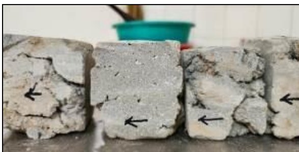
Fig -30: Core Samples taken. Print direction and top direction marked
