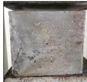
Fig -26: Cube crushed at 7 day & Cracking pattern studied
