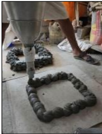
Fig -42: Extrusion process – Trial 02
