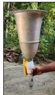
Fig -11: Concrete extruder fabricated with available resources
