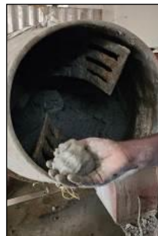
Fig -20: Trial Mix-01: Materials Mixed consistency checked
