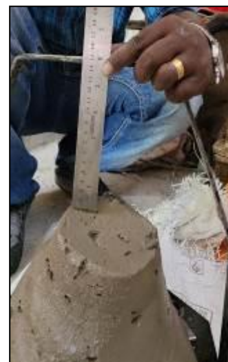
Fig -21: Measurement of Slump (Slump value observed =140mm)
