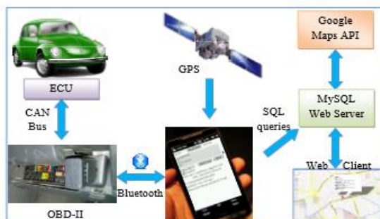
Fig. 7 Embedded software for tracking real time engines and vehicle signals.
