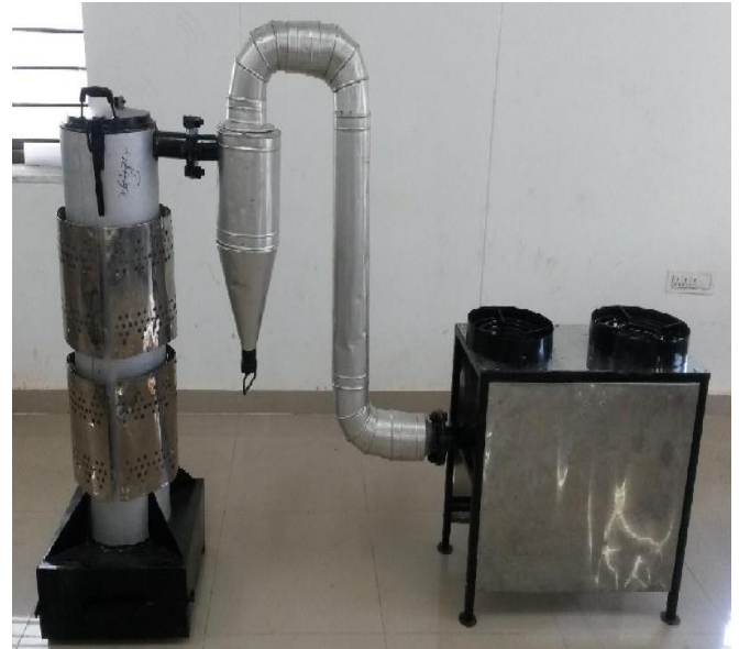
Fig.7 Assembly of the Updraft Gasifier
