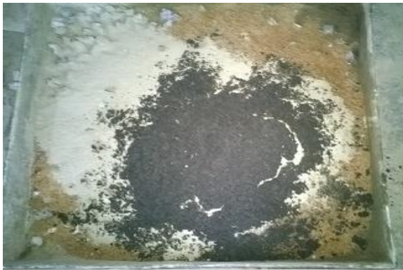
Fig. 2. Rice husk ash in concrete mix
