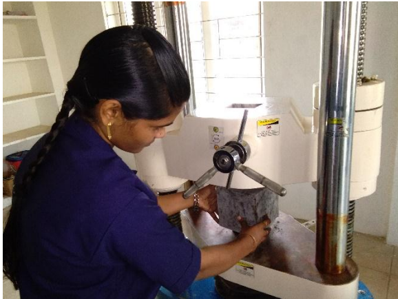
Fig1 conducting compression strength on cubes
