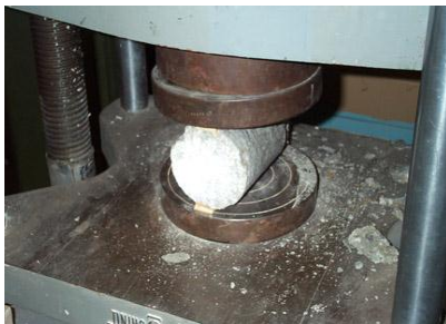
Fig2 conducting split tensile strength on cylinders
