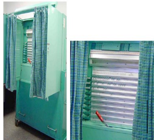
Fig 4: Mechanical lever based voting system [12]
