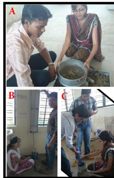
Figure 8 (A) Sieving of soil using 20mm and 4.75 mm IS sieve for preparation of sample. (B & C) Permeability testing by falling head method and Light compaction testing.
