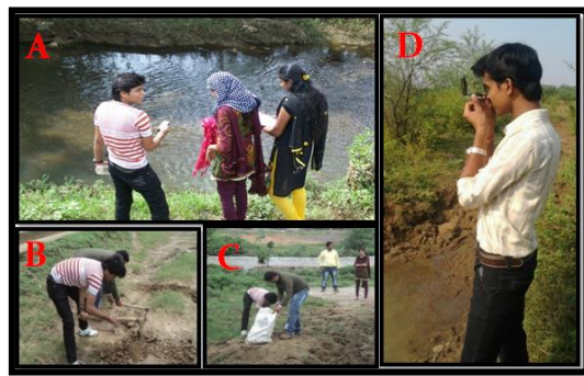
Figure 3 (A) Field photograph from the study area, while tracking satellite and taking coordinates and altitude data from Global Positioning System (GPS) instrument "Garmin etrex vista HCx. ( B & C ) The pictures of sites from where soil sample are collected and (D) Using clinometer at site for taking trend along stream.
