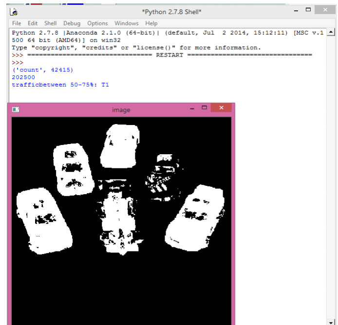
Fig. 3. Figure showing result of six cars detected and output showing 50=75% traffic
