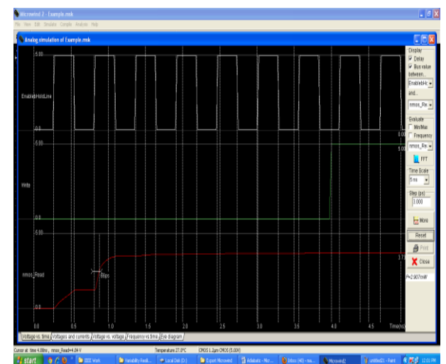
Figure -6: Characteristic waveform for Conventional 6T SRAM
