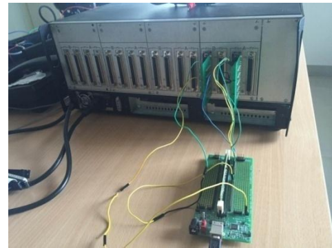
Figure 7: Hardware setup for hardware-in-loop simulation
