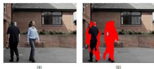
Figure 2.2: Temporal differencing sample. (a) A sample scene with two moving objects. (b) Temporal differencing fails to detect all moving pixels of the object on the left hand side since it is uniform coloured. The detected moving regions are marked with red pixels.
