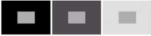
Fig 1.2: Simultaneous contrast .All the inner squares have the same intensity. But they appear progressively darker as the background becomes higher.
