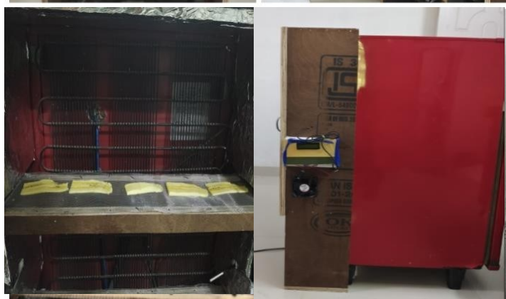
Insulated chamber fixed on refrigerator with circuit and fan
