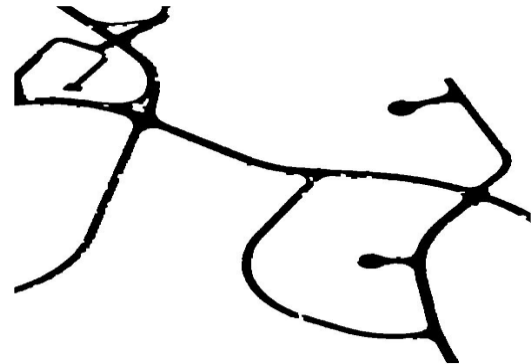
Fig13. Road network after shape based segmentation
