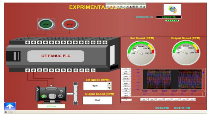
Fig 2.4 The view of the SCADA Experimental Screen
