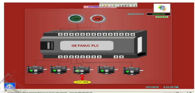
Fig 2.3 SCADA screen for controlling 5DC motors in an CNC machine
