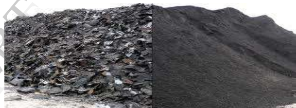
Fig 5: Shingles obtained before recycling and after recycling
