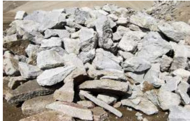
Fig 3: Concrete waste obtained after the demolition of a structure
