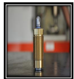
Fig (c) Hydraulic work support
