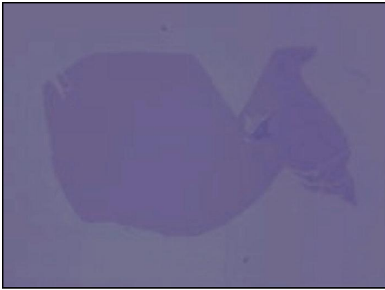
Fig 2: Monolayer graphene produced by mechanical exfoliation. Large sample with length of 1mm on Si/SiO 2 (reprinted from [6]; copyright 2012, International Scholarly Research Network ISRN Condensed Matter Physics).
