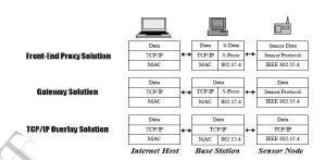
In front-end proxy solution, the base station serves as an interface between the data acquisition network (sensor network) and the data dissemination network (the Internet). The base station collects and stores all the information coming from the sensor network, and also sends any control information to the sensor nodes. There is no direct connection between the Internet and a sensor node: all incoming and outgoing information will be parsed by the base station [8].
