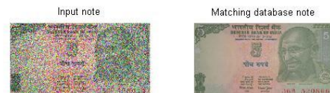
Figure 8. Recognition result of input note with gaussian noise (mean = 0 and variance = 0.05)
