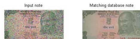
Figure 9. Recognition result of input note with salt and pepper noise (noise density = 0.1)
