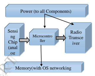
Figure 1.1 lists only the most important components of a WSN sensor. There could be other circuit parts depending on practical application requirements.for instance, we may plant a GPS receiver in a sensor to keep track of accurate positions to absorb solar energy.
