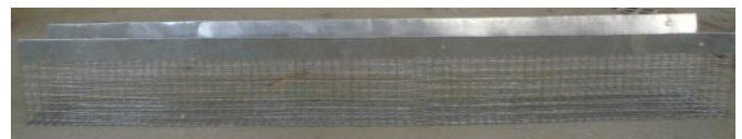
Fig. [1-a] Expanded galvanized steel wire mesh U-shape jacket with two straps at the ends.
