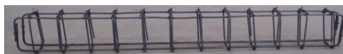
Fig. [4-a] Reinforcement details and location of internal mounted strain gauges for all tested specimens.
