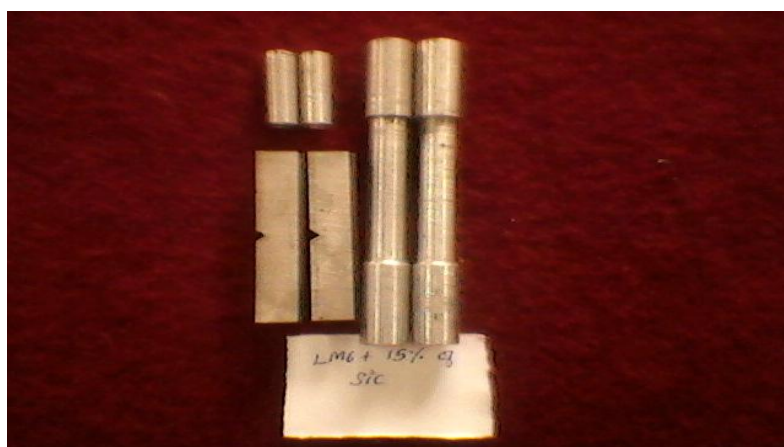
Fig.8(c). Tensile specimen with 15% of SiC in base lm6 alloy
