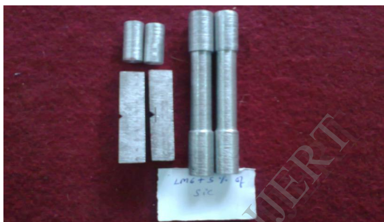
Fig.8 (b). Tensile specimen with 5% SiC in lm6 alloy
