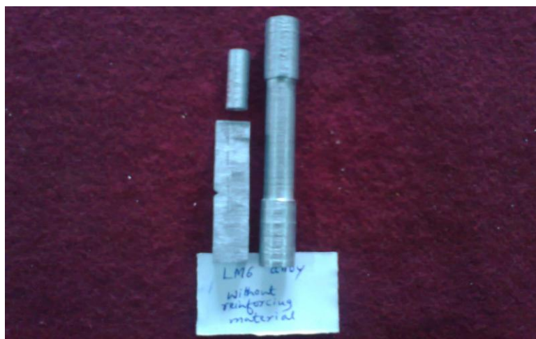
Fig.8 (a). Tensile specimen for base LM6 alloy
