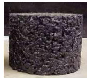
Fig. 4: Marshall compacted test specimen
