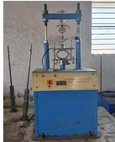
Fig. 3: Marshall Stability machine setup
