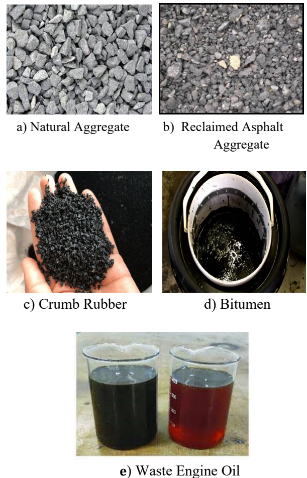
Fig. 1: Bituminous Mix Materials (a, b, c, d and e)
