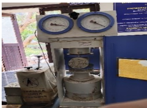
Figure 6: Cylinder under Split Tensile Testing Machine
