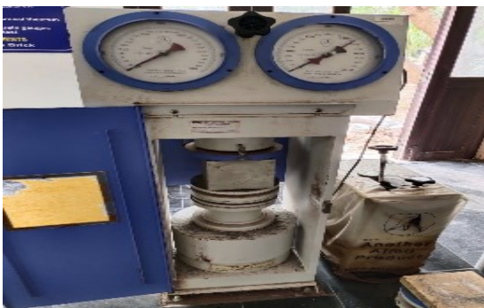
Figure 4: Cube Under Compressive Testing Machine
