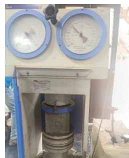
Figure 2: Cube Under Compressive Testing Machine
