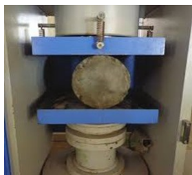
FIGURE 4: Cylinder Under Split Tensile Testing Machine
