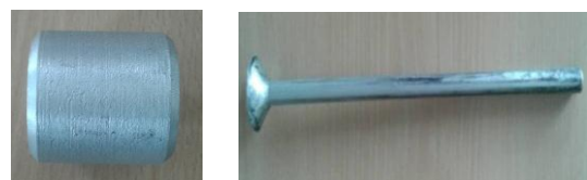
Fig 2.3: Extrusion Specimen (Before & After Extrusion Process)
