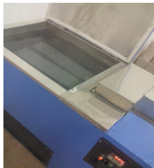
Fig 7:-Curing done with accelerating curing tank
