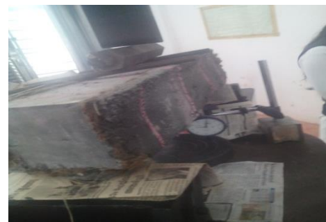
Fig 11:-Retrofitted beam tested for flexural strength in UTM
