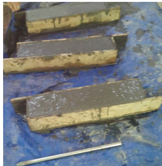
Fig 6:- Casting of beams
