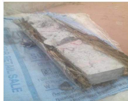
Fig 12:-Retrofitted beam after flexural strength test.
