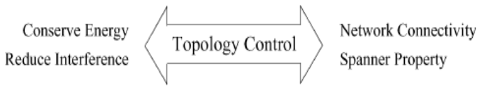
Figure-1: Topology control constitutes a trade -off between node energy conservation and network connectivity.
