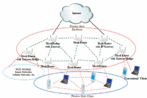
Figure 2: WMN Typical Structure
