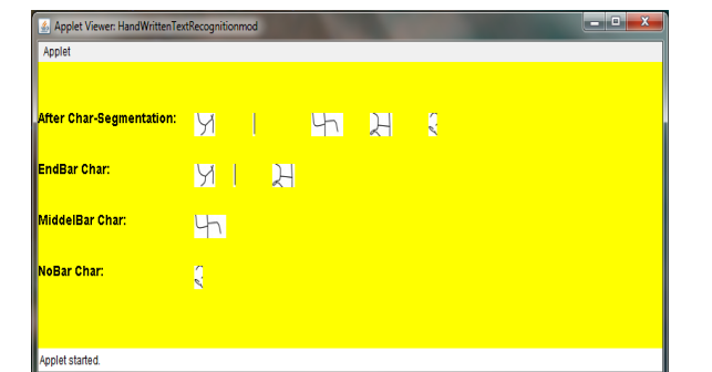
Fig.9 Identification and Separation of End Bar, Middle Bar and No bar Characters
