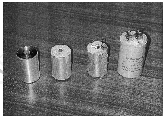
Fig. 1: From left: the coiled cylindrical element: the element with the sprayed ends; the element with the two connection wires; and the complete capacitor.
