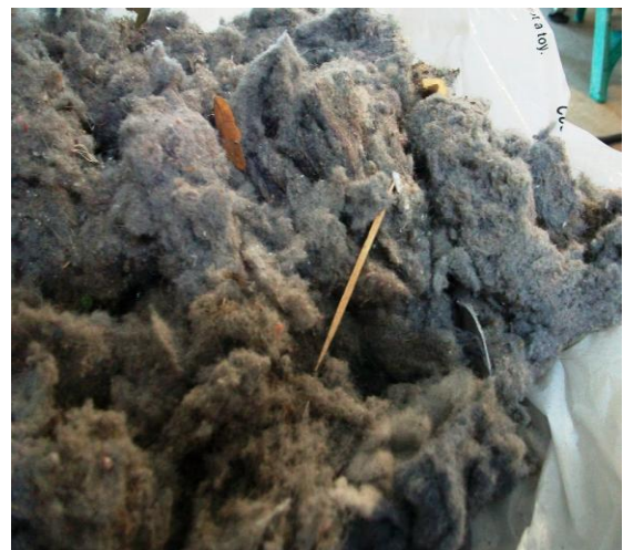
Figure 2. Fluff (as a waste material) obtained from tires.
