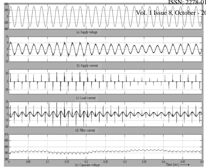
Fig. 2. Dynamic performance of PIAPF with the computer load. (a) Supply voltage (V). (b) Compensated supply current (A). (c) Load current (A). (d) Filter current (A). (e) Voltage across the dc capacitor (V).
