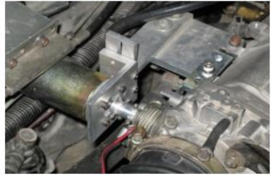
Fig.4. Drive-by-wire throttle valve system
