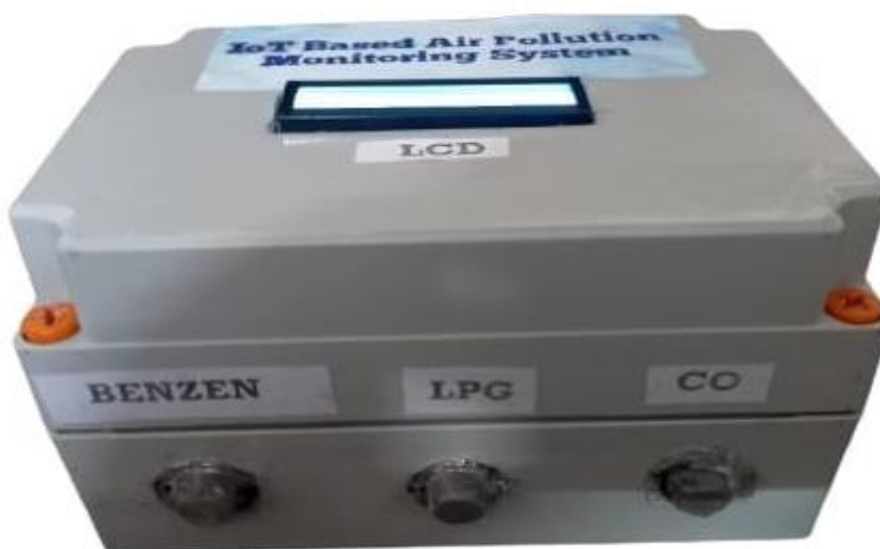
Figure 2. Actual Image of our IOT Based Air Pollution Monitoring System
