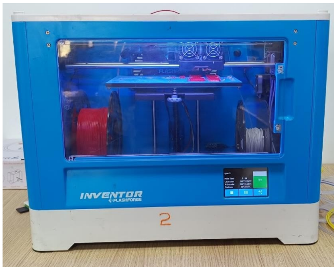
Fig. 1. Dual Extruder 3D Printer (FDM)
