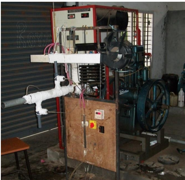
Figure IV.i: VARS Connected to Engine
