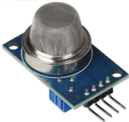
Fig -2: Gas Sensor
