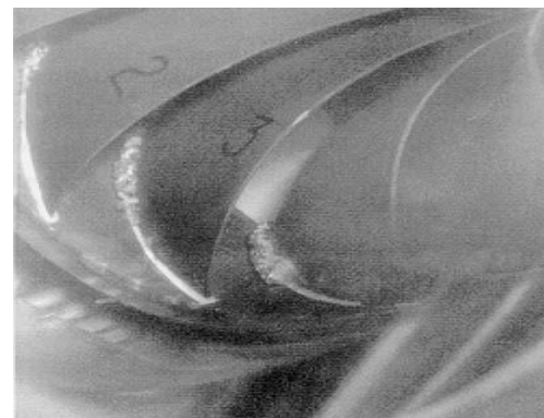
Fig1. Shows Leading edge cavitation Picture courtesy of Saini [22]
