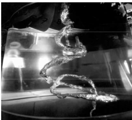
Fig 3.Shows draft tube swirl Picture courtesy of Saini [22]
