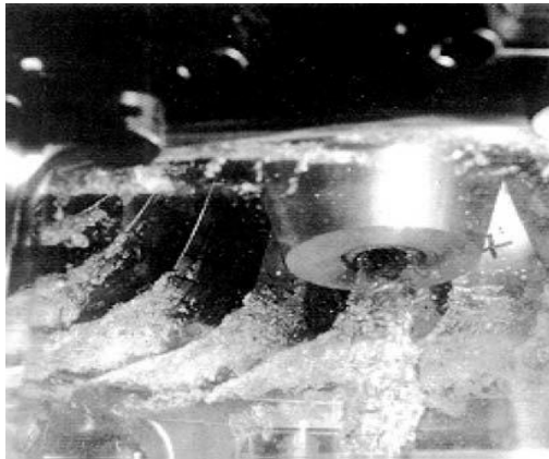
Fig2.Shows travelling bubble cavitation Picture courtesy of Grindoz [24]
