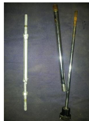
Fig.4. Removing clamping pipes from the triaxial cell and replacing with threaded MS rods
