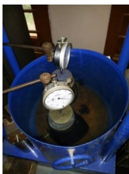
Fig.2. Immersing the samples under water and attaching the dial gauges to the center of the porous discs
