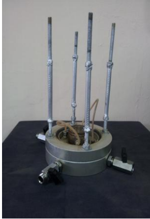
Fig.5. Permanently fixing the cell ring to the base using threaded MS rods and nuts.
