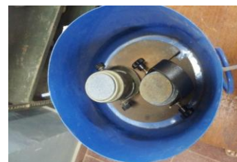
Fig.1.Preparation of samples enclosed in rubber membrane, confined by the split sand former.
