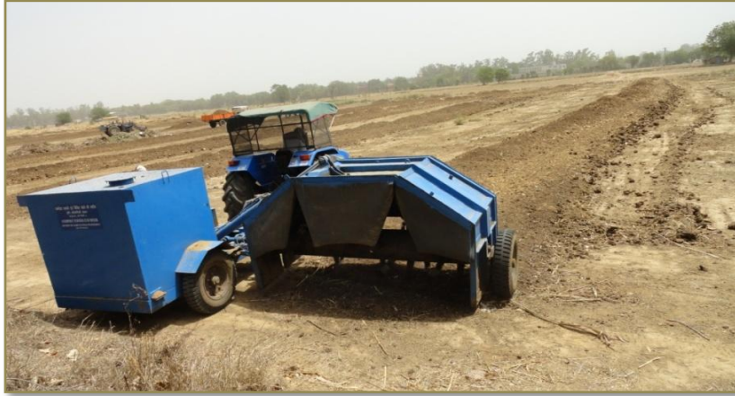
Picture 2: windrow turner for mixing materials uniformly
