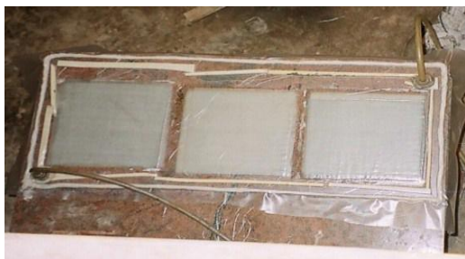
Fig 1: Vacuum bagging process
