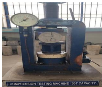
Figure 8.3 Split Tensile test
