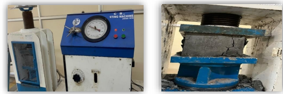
Figure 2: Compressive Strength Test on Cubes
