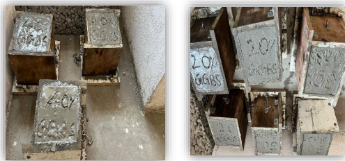
Figure 1: Casting of Cubes
