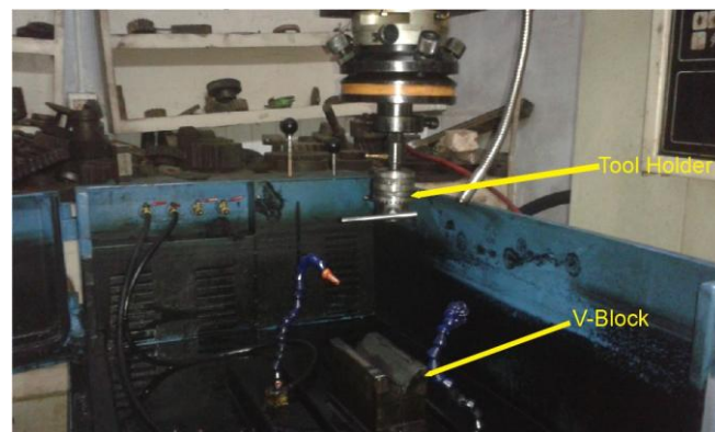
Fig.6 V-Block and Tool Holder arrangement
