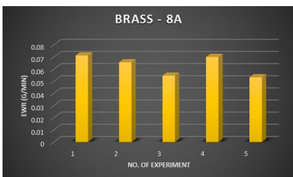
Fig.17 Electrode wear rate at 8A
