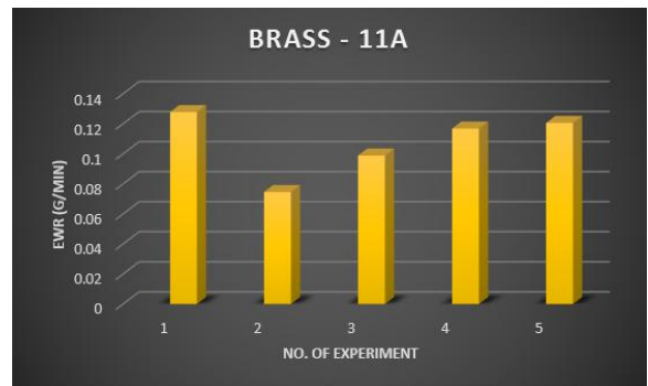
Fig.18 Electrode wear rate at 11A
