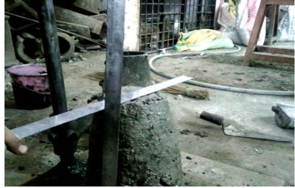
“Figure 4.1 Measurement of Slump of concrete mix”
