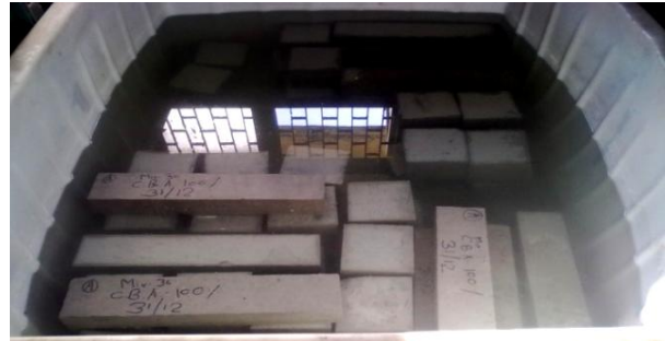
“Figure 3.2 Curing tank with cubes and beams”
