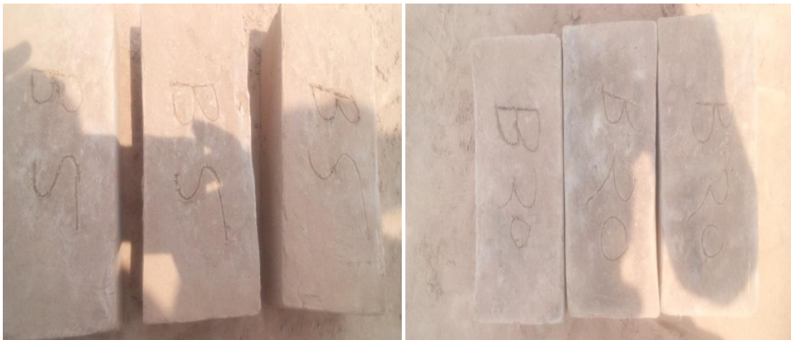
Figure 6. Rice husk ash bricks and bagasse ash bricks before testing
