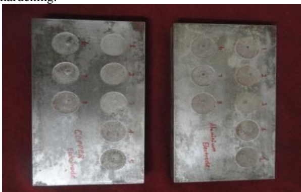
Fig 3.1 OHNS Die Steel (Work Piece) after machining
