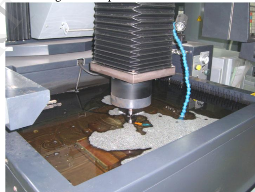
Figure 4.2 EDM tank with electrode and work piece
