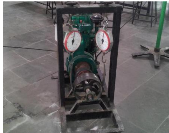
Fig.1: Single cylinder 4-stroke diesel engine setup
